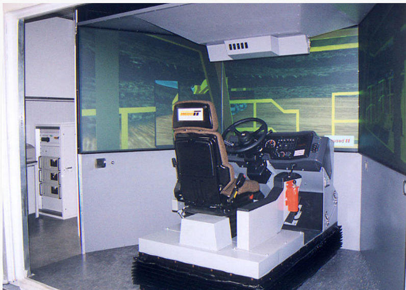
First Advanced Equipment Simulator for the mining industry - AES Series 1
