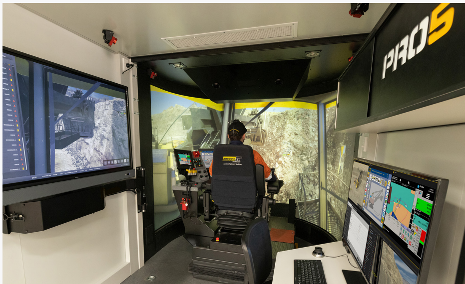
PRO5 - Advanced Equipment Simulator equipped with 3D stereoscopic display and professional grade visual system
